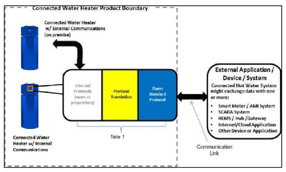
**Connected Water Heater Communications Architecture**
