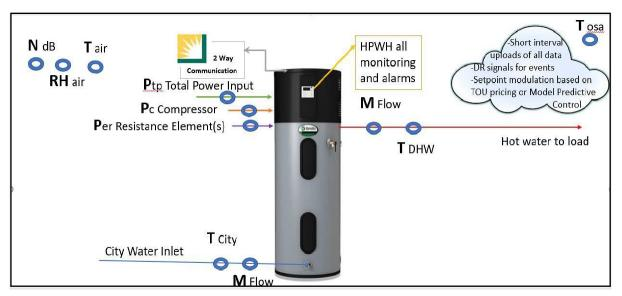
Metering Diagram for HPWH Performance Testing
