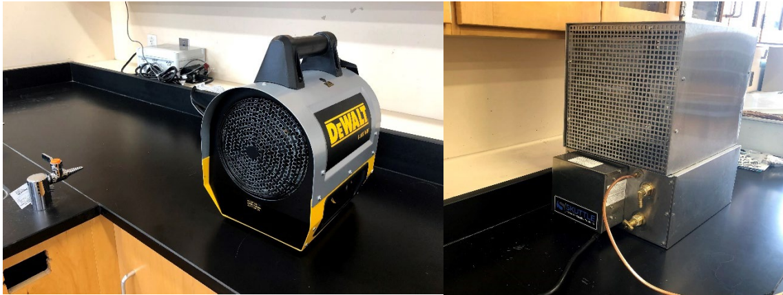
FIGURE 9. HEATER (LEFT) AND STEAM HUMIDIFIER (RIGHT) USED TO SIMULATE LOADS IN CLASSROOMS DURING SCHOOL CLOSURE.
