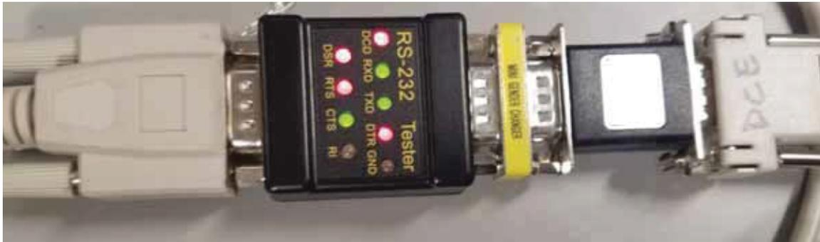
Figure 7. Successful RS-232 Testing Setup Used with Vendor B's Radio and the Meter
