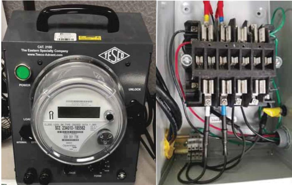
Figure 2. Meter Sockets Used for Testing
