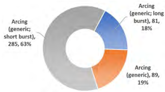
Figure 14. ECCVM Recorded Shunt-Arcing Events by Type
