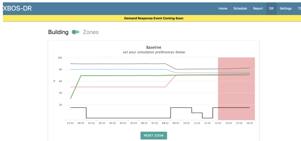
Figure 5: Display of Simulated Data on DR screen of User Interface
