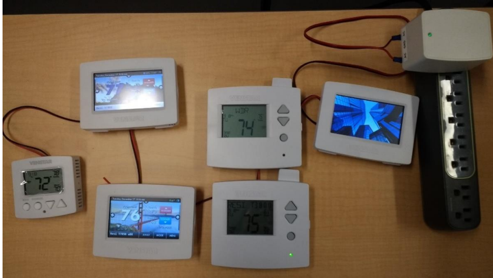
FIGURE 1. VENSTAR THERMOSTATS TESTING SETUP
