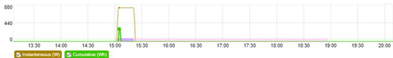
FIGURE 18: HOME 3 WATER HEATER RESPONSE TO A “LOAD UP” EVENT
