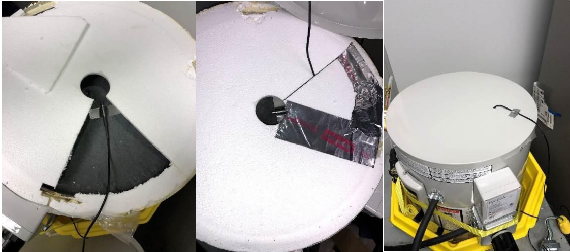
Figure 28 – Temperature Probe Install on Water Heater
