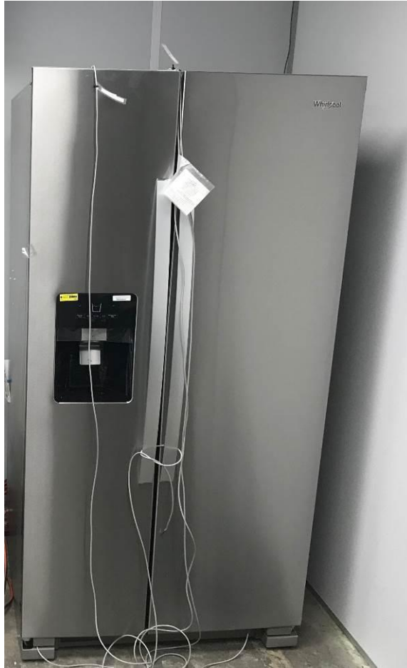
Figure 17 – Refrigerator with Temperature Probes
