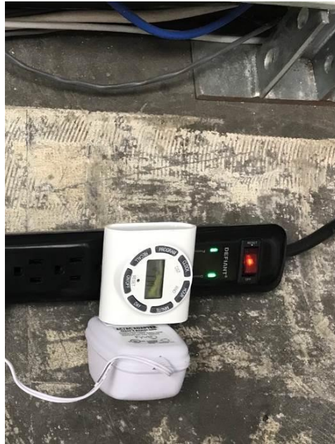
Figure 44 – Timer and 24 VAC Source to Simulate AC Cycling
