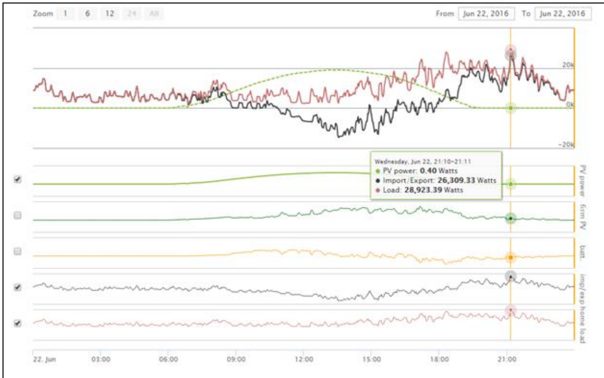
Figure 6-4 Aggregated operation of storage in a group of homes equipped with battery storage
