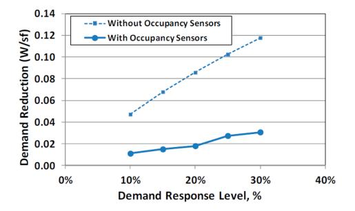
Figure 2: Demand Reduction with and without Occupancy Sensors
