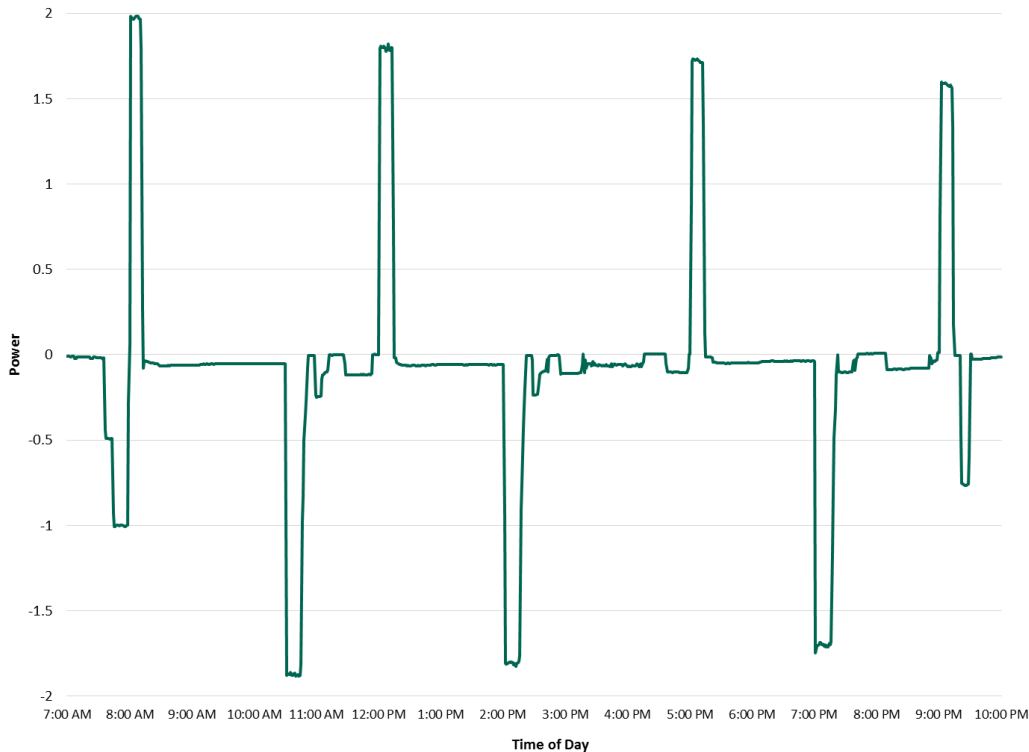
Figure 69: DBESS Charge/Discharge Profile (October 24, 2014)
