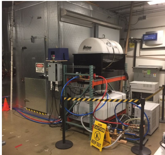
FIGURE 29. CCEL DAQ AND CONTROLS (TOP LEFT), WATER HEATER TEST UNIT (TOP RIGHT), AND WATER HEATER TEST RIG (BOTTOM)
