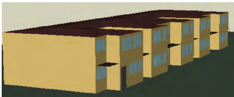
Figure 18: Built-Up Energy-Plus Model of 10-Unit Apartment Building
