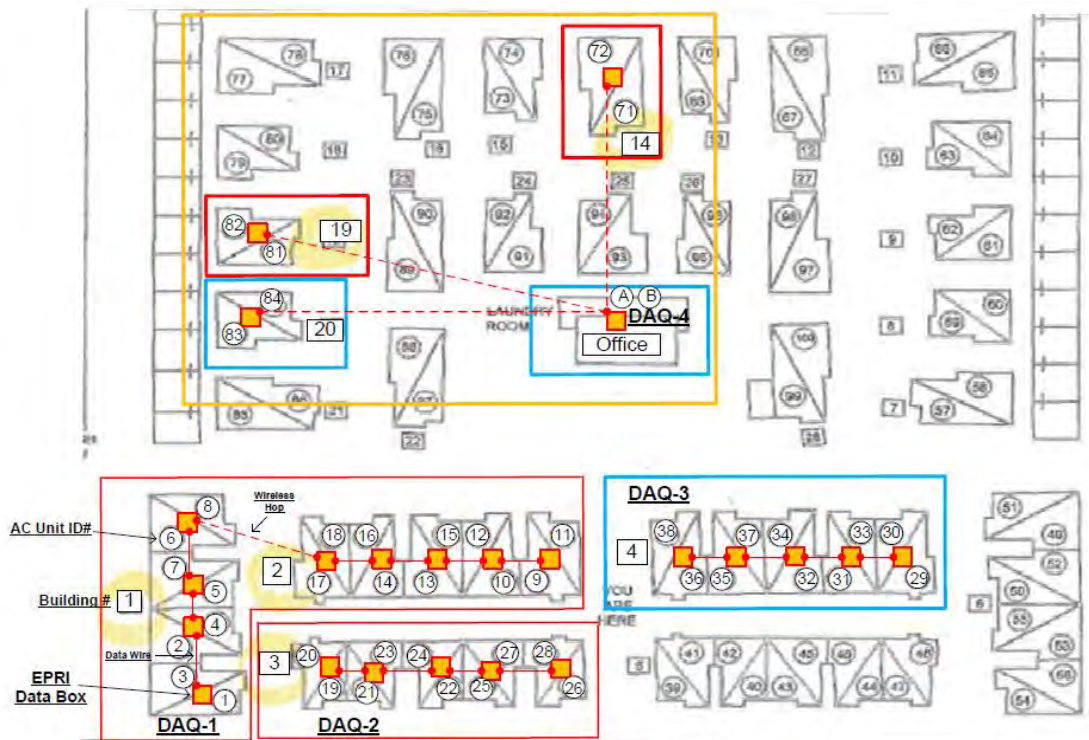
Figure 32: Overview of EPRI Data Acquisition System Layout
