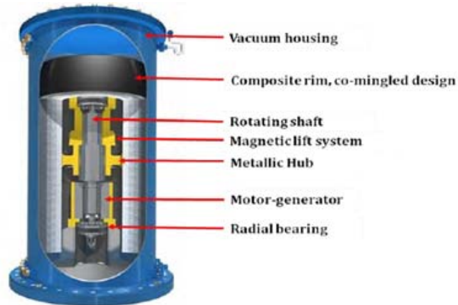
Beacon Flywheel Primary Components, 100 kW & 25 kWh model
