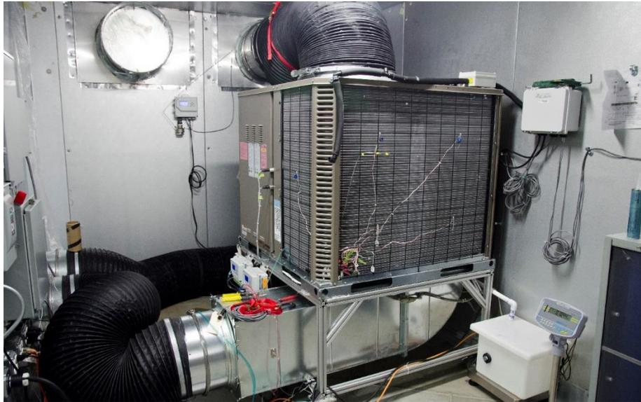
**FIGURE 6: TEST UNIT INSTALLED IN THE ENVIRONMENTAL CHAMBER**
